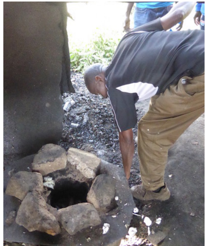
Above: Energy-efficient jua-kali stove using waste woodchips to cook crisps sold by street vendors.
