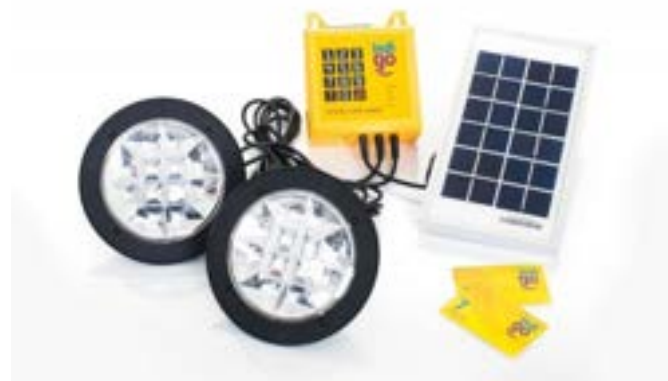
Figure 70: Picture of a solar home systems kit (Collings, 2016).
